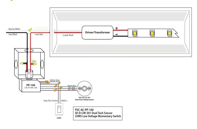
Wiring Example Application: Controller Installed In Electrical Enclosure, Network Application
