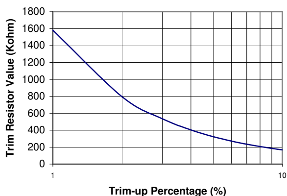
Fig. 19 Trim-Up Resistor Selection
