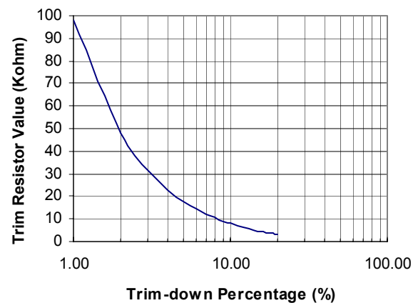
Fig. 18 Trim-Down Resistor Selection
